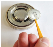
Optional analysis plates allow to collect particles in the impactor of the HT-HR-ELPI®+ in 14 separate size fractions for later microscopical or chemical analysis
