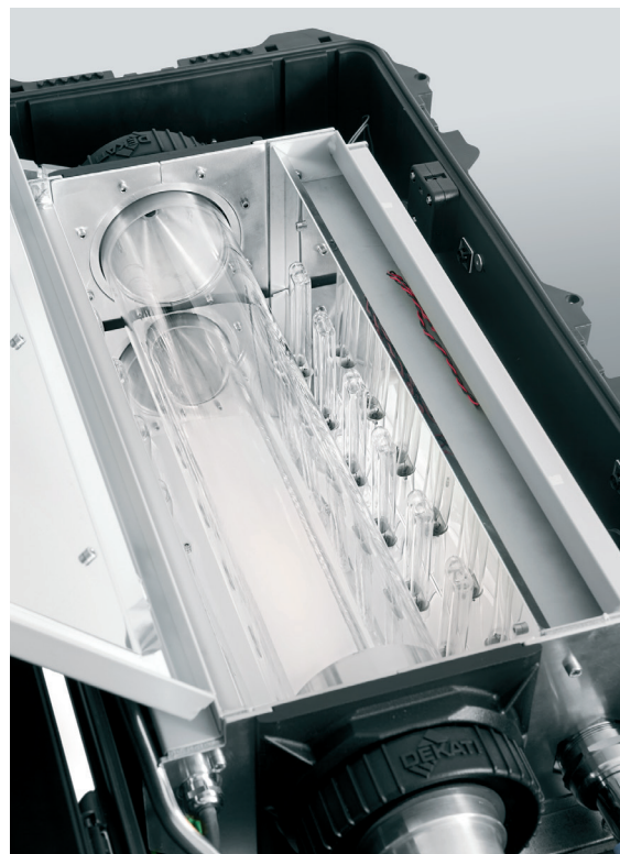
DOFR™ oxidation chamber is made of clear glass and surrounded with 12 UVC lamps operating at 254 nm.
