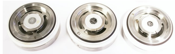
HT-DLPI+ and HT-ELPI®+ collect particles in different size fractions on 25 mm filters
